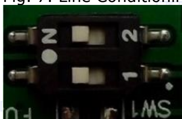
Fig. 7. Line Conditioning Jumper
